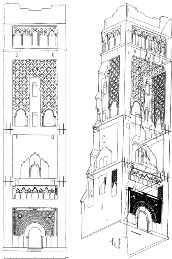
Figure 9. Elevation and 3D model of the minaret of Mansura
